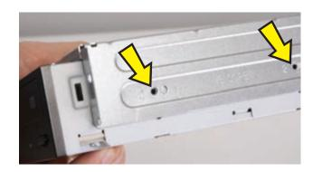
3 Replace the four drive cage screws.
